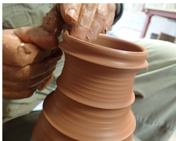
Figure 19. Forming a collared rim on the potter's wheel by holding certain finger positions.
