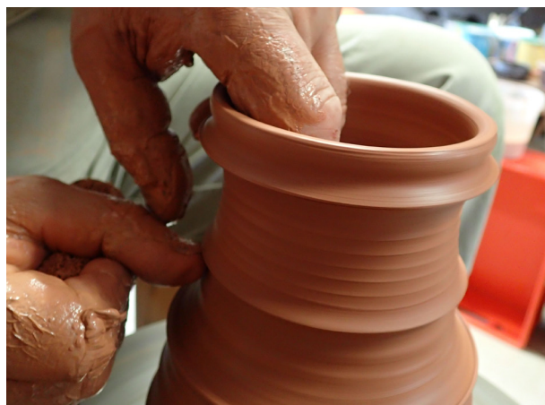
Figure 25. Johannes Klett-Drechsel creates horizontal corrugations and strips while throwing a jug.
