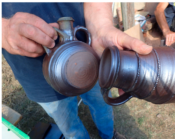
Figure 14. During kiln firing, vessels stacked on top of each other show clear differences in colour at the contact points. In the covered area, the engobe is hardly sintered and of a significantly lighter colour.
