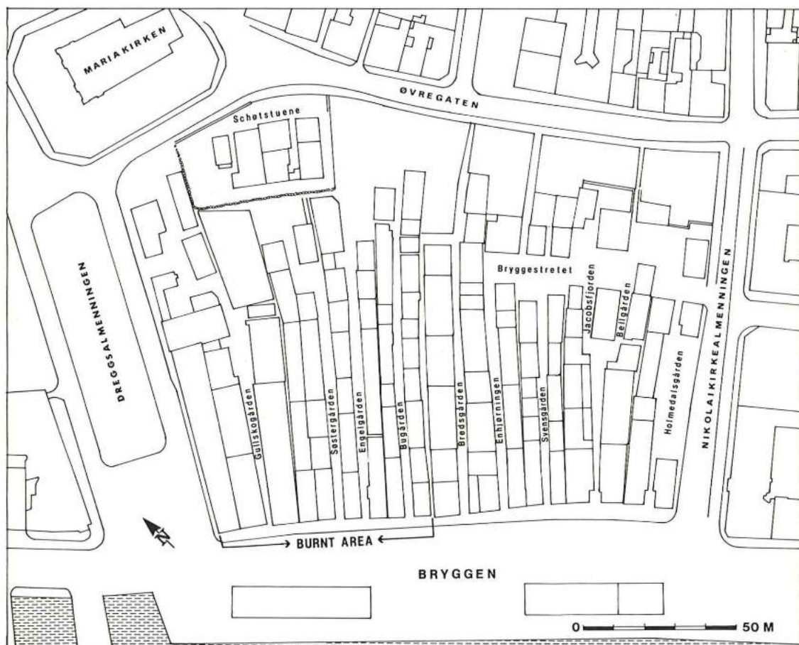
Fig 3 Sketch-plan of the Bryggen complex before the 1955 fire. Of the burnt-out properties, Bugården and Engelgården were regular double tenements with a passageway between the two house-rows. Søstergården's passageway ran up the south side of the tenement (next to Engelgården), and Gullskogården had acquired a third row of houses to the north, with brick facings
