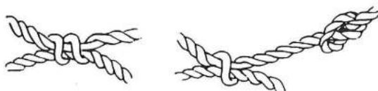
Fig 39 The binding technique of the net fragments found at Bryggen. Illustration from Schjølberg 1988
